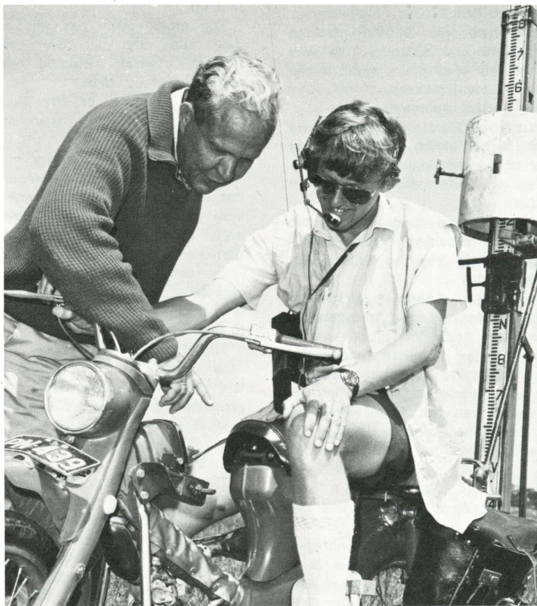
Hart, left, checks the odometer on the special motor-cycle before his assistant, Len Eacott, takes off on a survey run.
